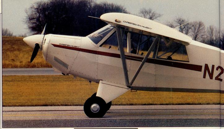
Most of the high-wing fabric airplanes designed in the 1930s—the Cub, Taylorcraft, Champ, Porterfield and Interstate—have virtually identical wings, according to Andersen: Clark Y or USA 35-series airfoils with a 63-inch chord, 35- to 36-foot span and 6.66:1 aspect ratio. What are the vital statistics for the Husky wing? Modified Clark Y-USA 35B airfoil, 63-inch chord, 35.5-foot span, 6.66:1 aspect ratio.
