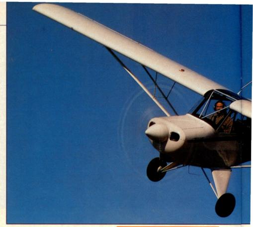
per Cub: Right foot on step, right hand gripping tubular brace over panel, swing left leg over seat and control stick, settle into seat. Exit by hoisting yourself out of the seat so you can sit on the door frame and swing both legs out of the cabin.
